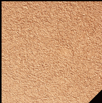
DELTA Delta Finish utilizes approximately 1.5 mm quartz aggregates and can be floated to create a medium sand finish or troweled to achieve a lace texture.
