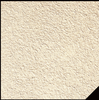
OMEGAFLEX MEDIUM OmegaFlex Medium Finish utilizes approximately 0.8 mm quartz aggregates and can be troweled or floated to achieve a medium sand finish.
