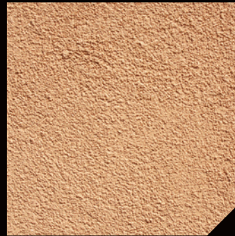
MALIBU Malibu Finishes utilize quartz aggregates and come in the following options: Malibu 12 (~1.5 mm): Coarse sand finish with slight worm driven appearance. Malibu 16 (~1.2 mm): Medium sand finish with slight worm driven appearance. Malibu 20 (~0.8 mm): Fine sand finish with reflective quartz aggregate. Malibu Fine (~0.8 mm): Imperfect smooth type finish with irregularities. (Malibu 16 pictured)
